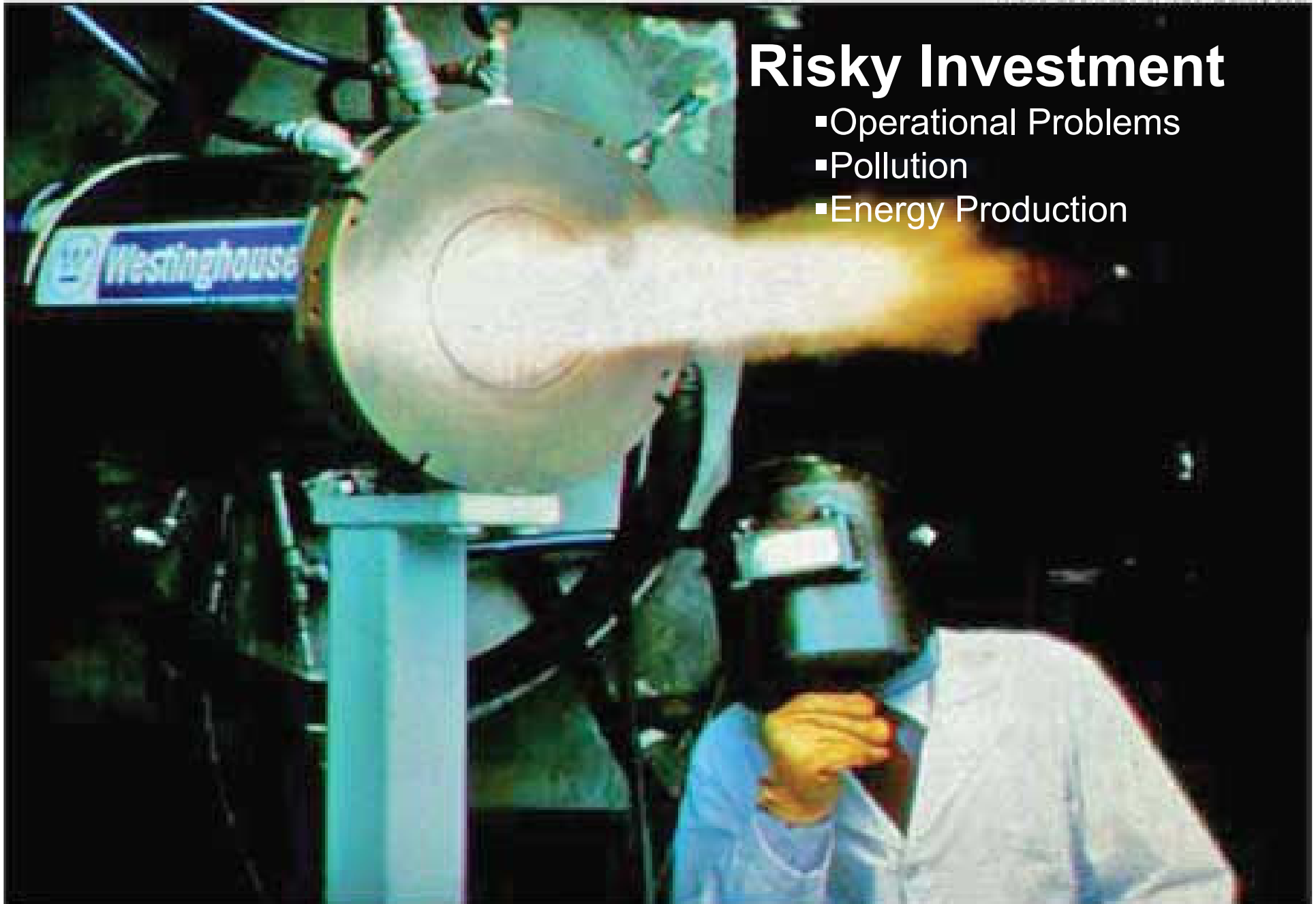
The plasma-heating unit creates the plasma arc used to turn trash into gas and rock-like material.
